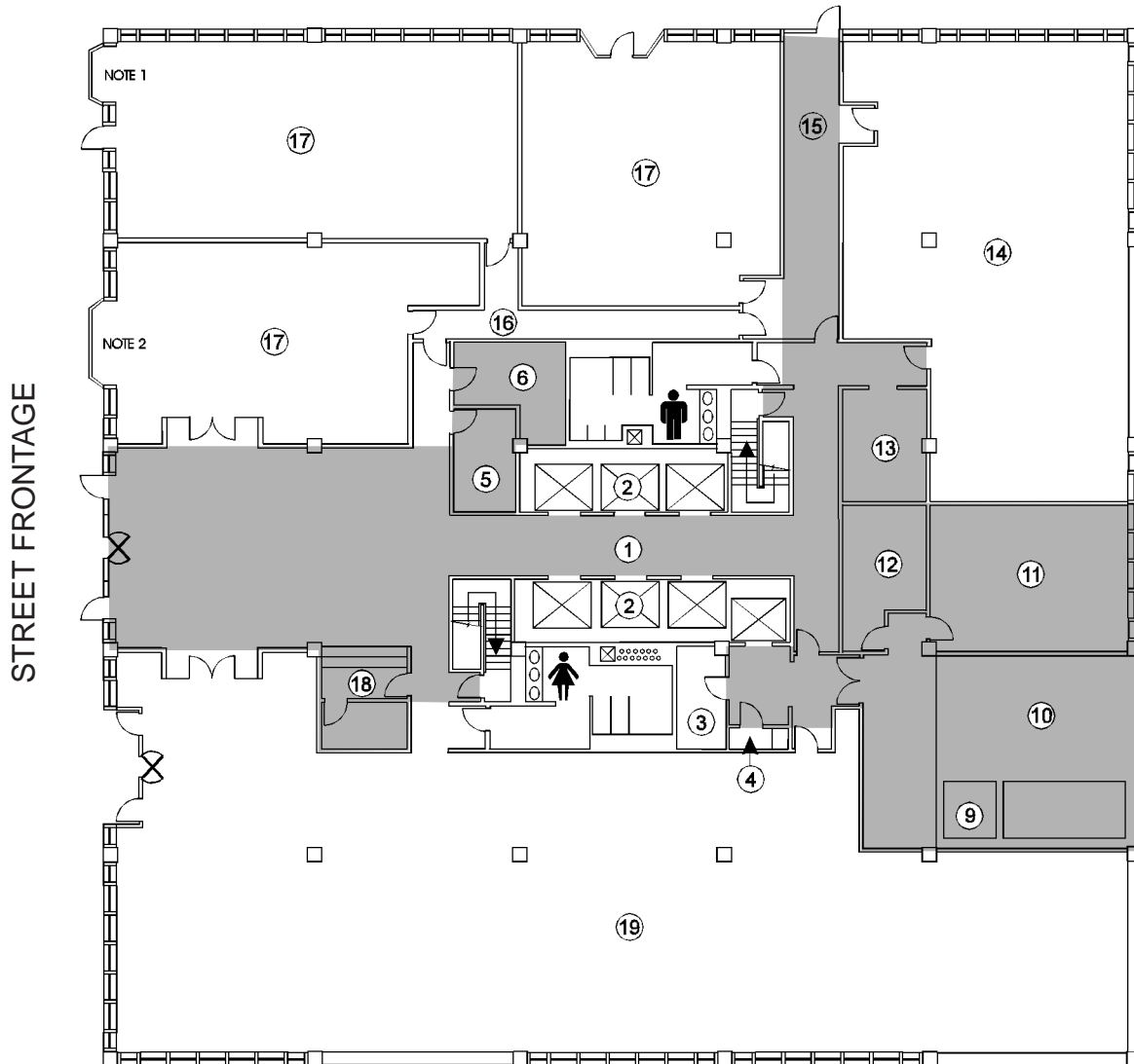
ILLUSTRATION OF BUILDING COMMON AREA FOR A TYPICAL GROUND LEVEL FLOOR WHERE THE BUILT AREA BOWS OUT OF AN OTHERWISE STRAIGHT BUILDING LINE (Note 1) AND A BAY WINDOW EXTENDS OUTSIDE THE BUILDING LINE (Note 2)
